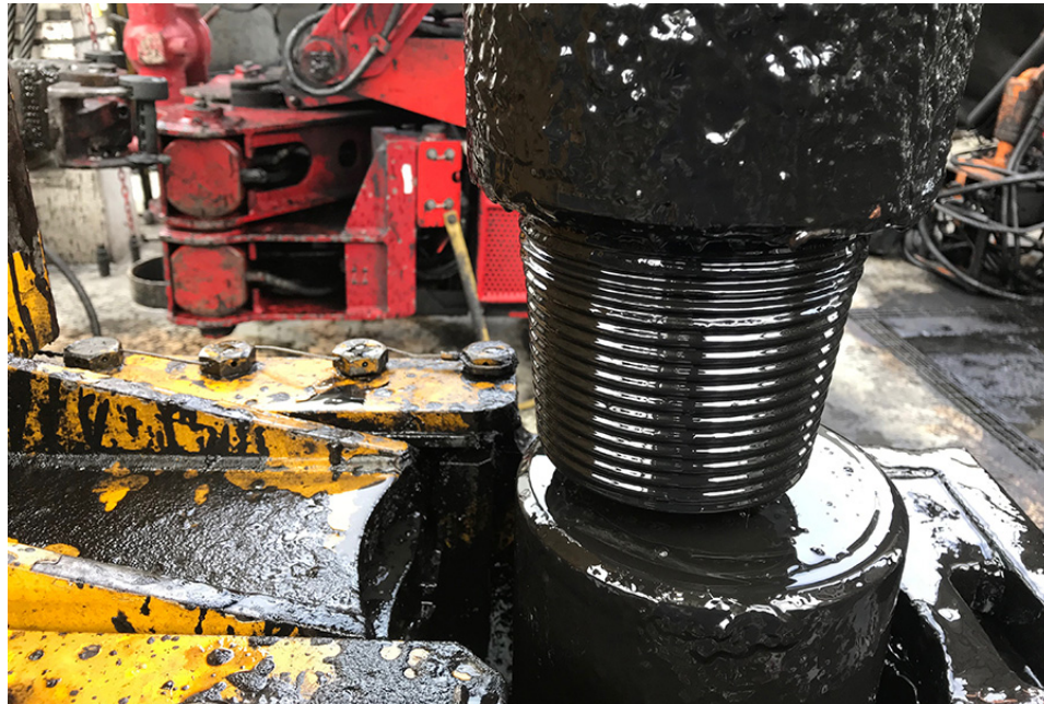
Figure 1: Quill not Aligned with Well Center
